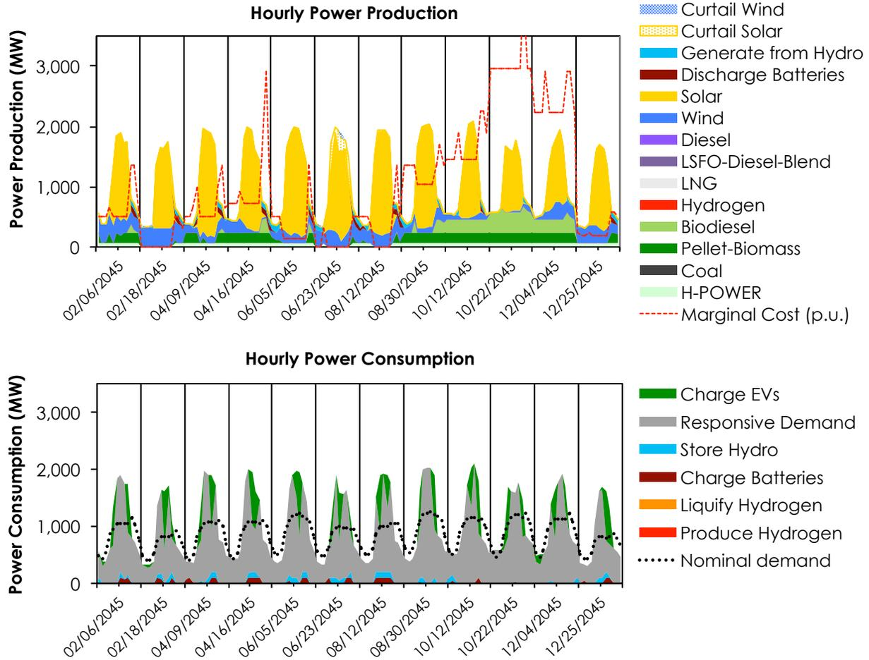
**Figure 3. Hourly power production and consumption on Oahu during 12 sample days in 2045, with 100% renewable power**
