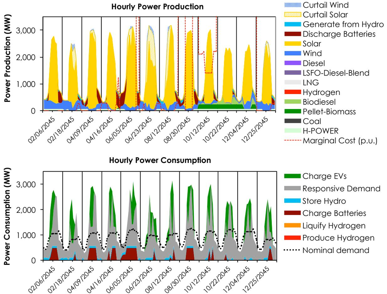
**Figure 4. Hourly power production and consumption on Oahu with 100% renewable power and biofuels limited to 5% of production**
