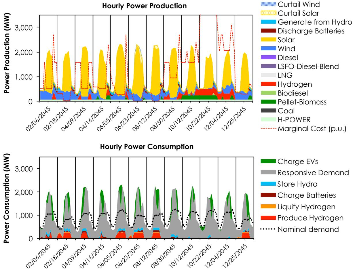
**Figure 5. Hourly power production and consumption on Oahu with 100% renewable power, biofuels limited to 5% of production, and an option for hydrogen energy storage**
