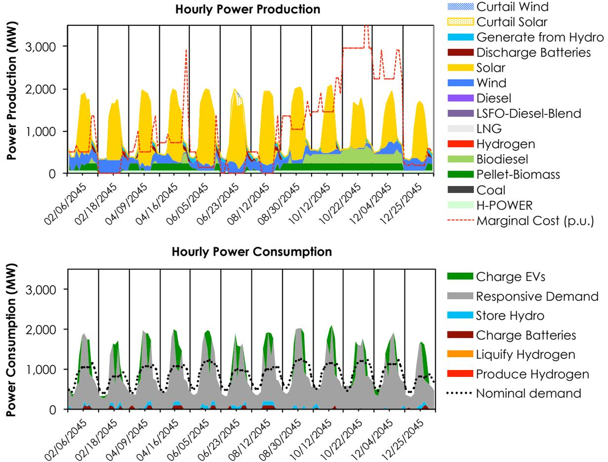
**Figure 3. Hourly power production and consumption on Oahu during 12 sample days in 2045, with 100% renewable power**
