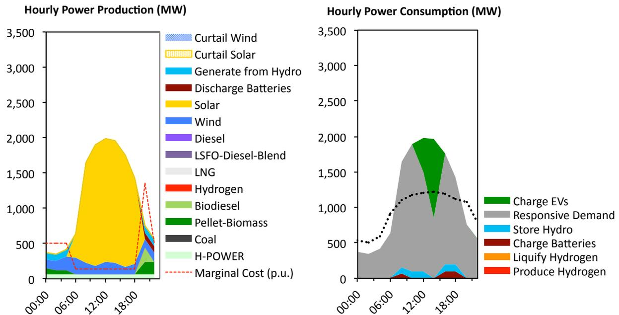
**Figure 2. Hourly power production and consumption on Oahu during an April day in 2045, with 100% renewable power**
