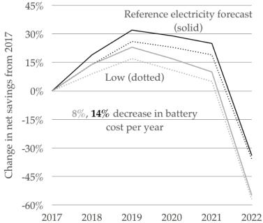
Figure 3. Potential change in net savings compared with 2017. Solid lines reflect reference electricity prices and dotted lines reflect the low electricity price forecast. The upper dark lines correspond to a 14% decrease in battery cost per year, and the lower gray lines reflect an 8% decrease.
